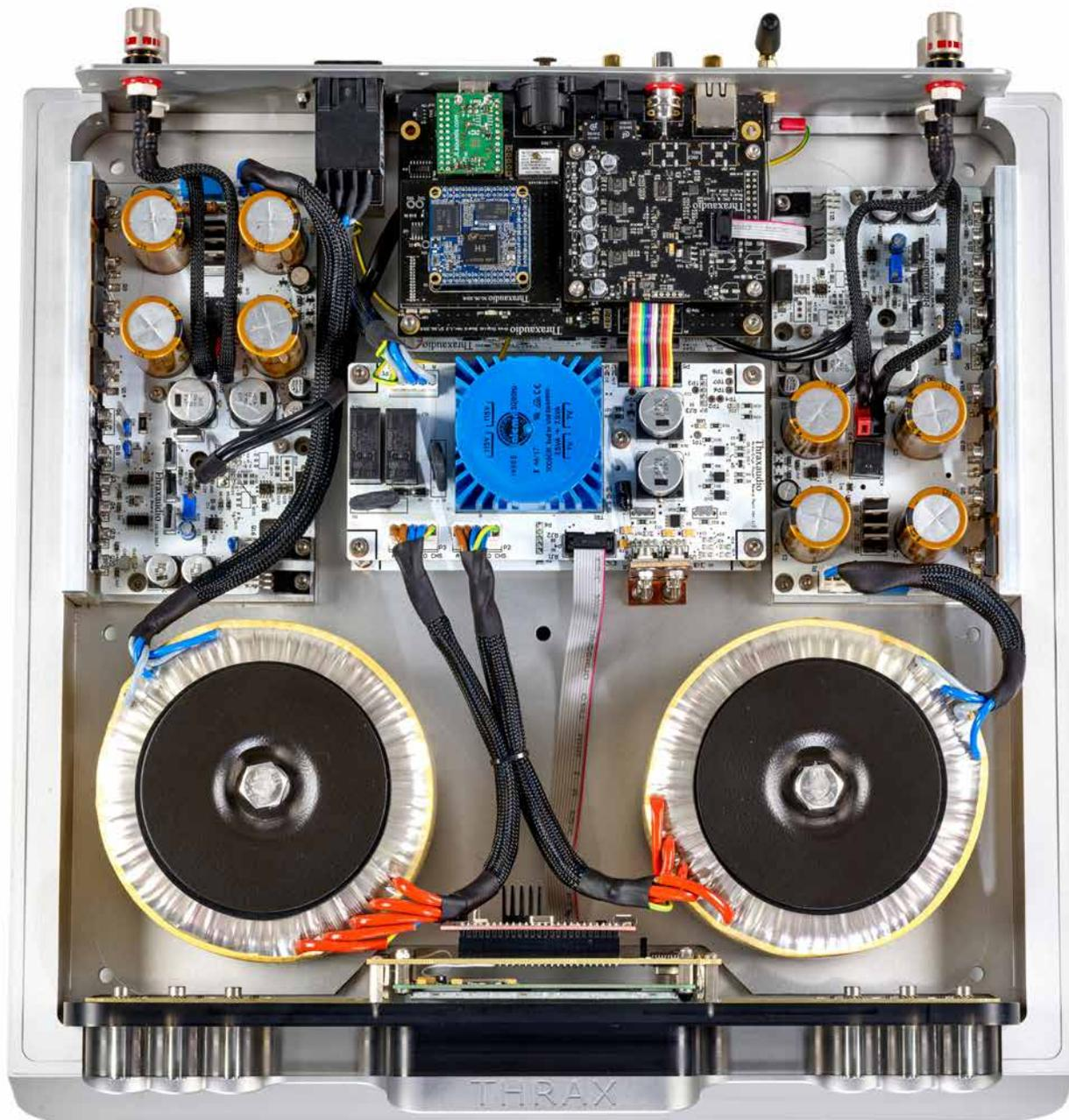
The bulky housing walls (that make the amplifier absurdly heavy) leave less room inside than you might think. However, Thrax perfectly utilizes the available space: the signal path is clearly identifiable, from the central current control through to the transformers and the identical monos (right and left).
