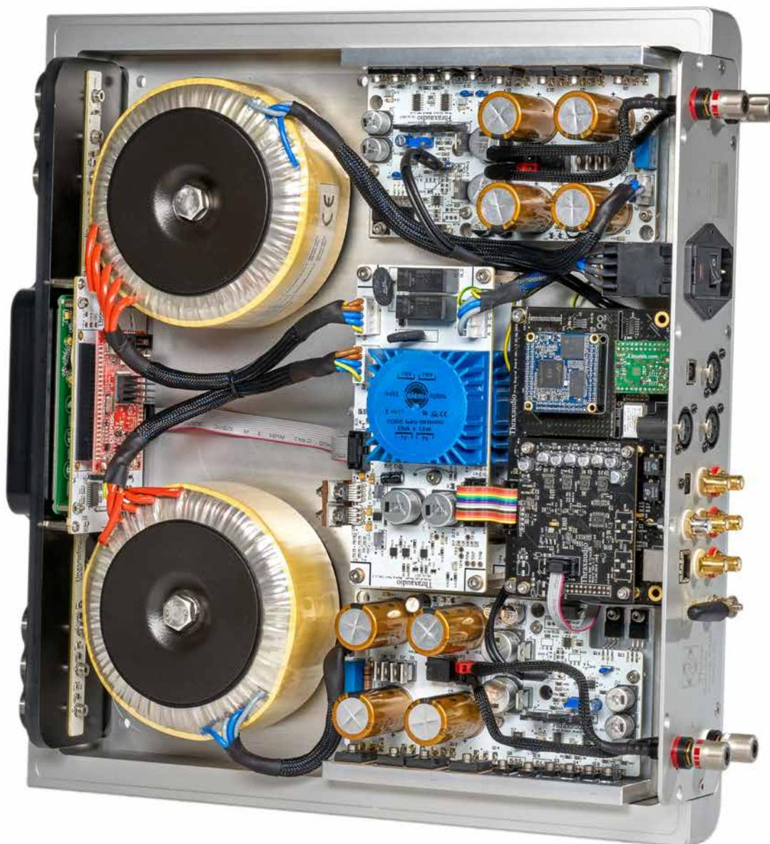
Preamplification and input selection are located right beside the rear housing wall. Almost all functions (DAC, streamer, Bluetooth, USB etc.) are housed on their own circuit boards in the modular design. This means that upgrades and straightforward repairs can be easily conducted.
