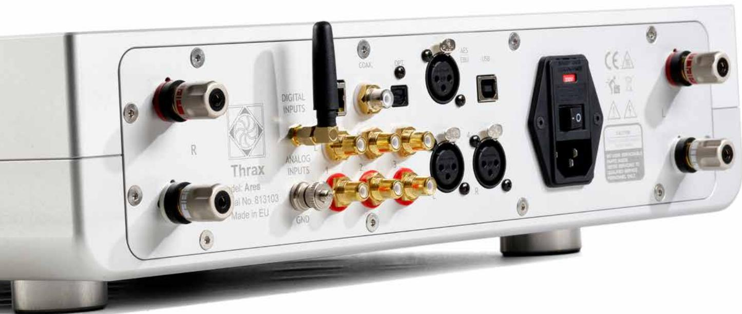
At first, the back side seems a bit busy, but it's actually well organized: on the top is digital (3 x S/PDIF plus LAN and USB), on the bottom is analog (3 x RCA incl. phono and 1 x XLR). Furthermore, the loudspeaker outputs are arranged with so much room that any terminals, be they bananas or even cables as thick as your arm, can be connected without any problems.
